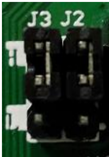
High speed mode: Short-circuit the upside 2 pins of JP2&JP3's with Caps.
