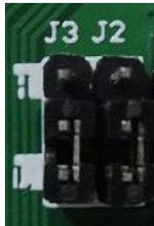
Low speed mode: Short-circuit the downside 2 pins of JP2&JP3's with Caps.
