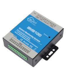
•Can measure 12 way basic voltage, 1 way total voltage; support 12 sections of 2V, 6V, 12V single battery voltage monitoring, total voltage Max. 300VDC;
