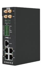
•4G, Ethernet WAN, WLAN WAN link switching and ICMP detection; •Support IPsec/OpenVPN/L2TP and other VPN; •WiFi support AP and client modes (2.4GHz); •1 x WAN, 3 x LAN, RJ45 interface type, 10M/100Mbps, self-adaptive MDI/MDIX: •Equipped with 2DI, 2DO, 4AI; •1 x RS485,1 x RS232, Support command mode and Transparent trans-
